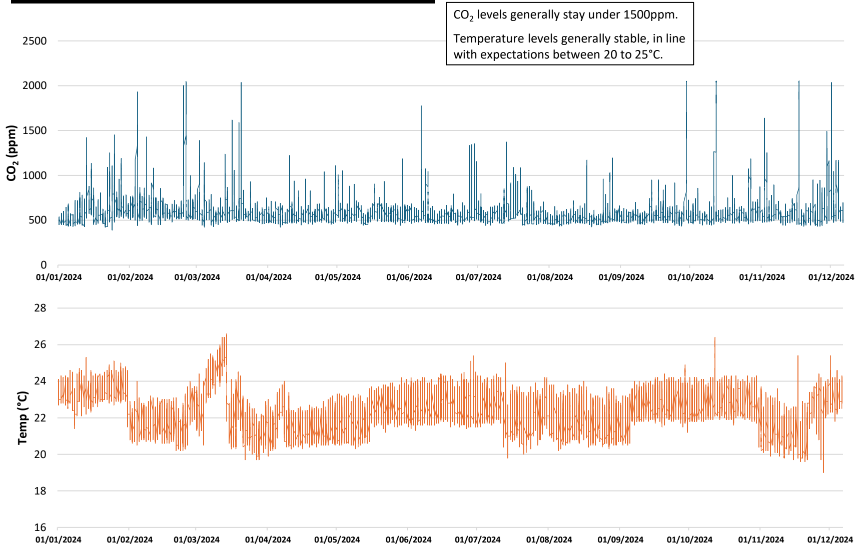
Figure 5: The internal conditions in Hall 3 from January 2024 to end of November 2024.
